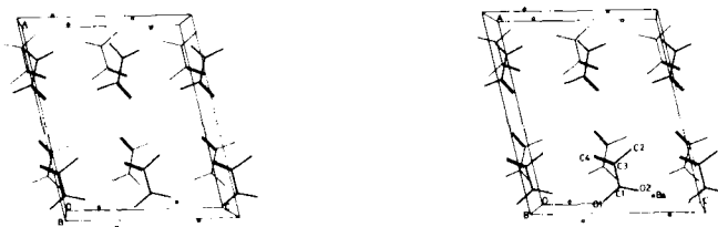
FIG. 4. Stereoscopic view of the packing of barium methacrylate anhydrate in the cell viewed down the a axis.
